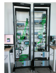
Real-time control system: Siemens PLC 1500/1200
